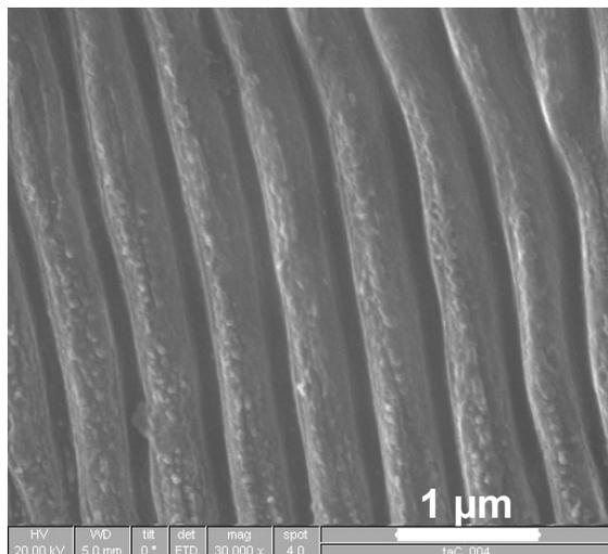
**Fig. 1:** Scanning electron microscope image of generated ripple-structures on an 1,5 µm thick ta-C-layer.
