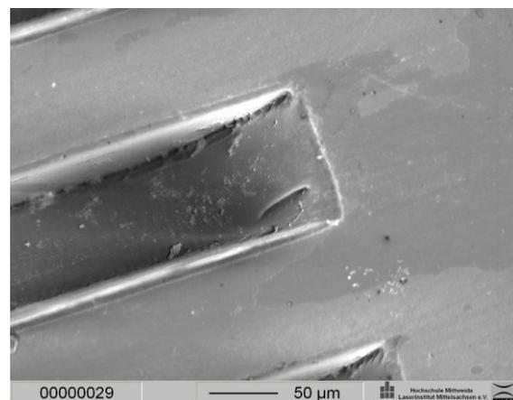
**Fig. 3:** SEM image, microstructures in polystyrene, bar wide and groove wide 100 µm, depth of structure 50 µm.
