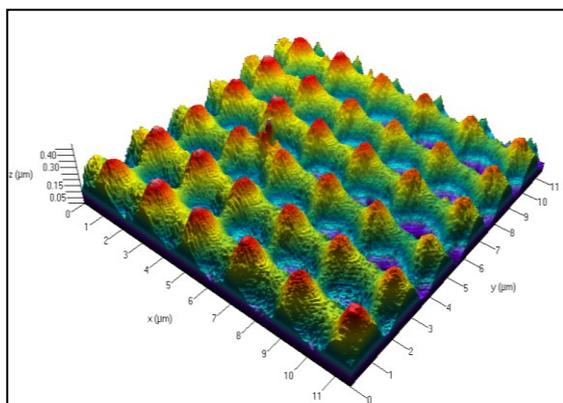
**Fig. 5:** Laser scanning microscope image, microstructures in a 1,5  $\mu\text{m}$  thick ta-C-layer, average distance of burling 2  $\mu\text{m}$ , depth of structure ca. 300 nm.
