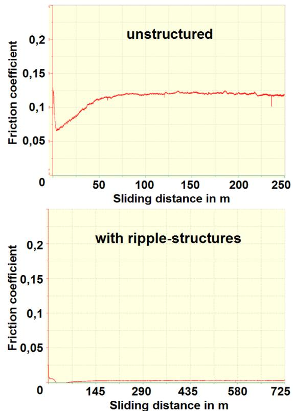
**Fig. 2:** Results of tribometer tests for determination of friction coefficient on a ta-C-coated steel probe (testing method: ball on disk; ball: 100Cr6,  $\phi$  6 mm; load: 1N; top: unstructured ta-C-layer; down: ta-C-layer with ripple-structures).
