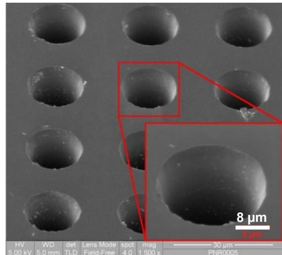
**Fig. 6:** Array of drillings in fused silica with a distance of 30  $\mu\text{m}$ , a drilling diameter of 16  $\mu\text{m}$  and an average depth of 50  $\mu\text{m}$ .
