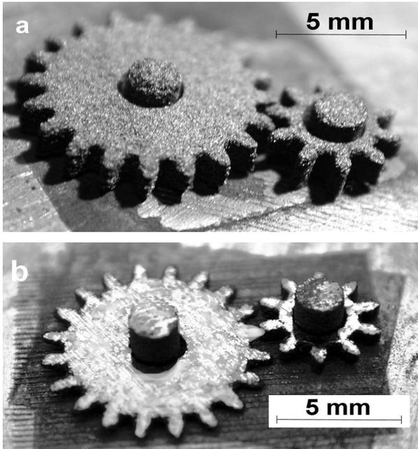
**Fig. 2a:** laser micro sintered gear wheels (steel 1.4404, normal atmosphere). **b:** gear after finishing.
