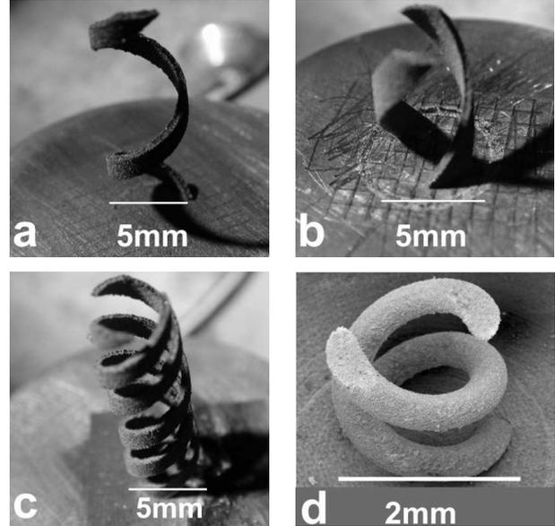
**Fig. 4a,b,c:** single, double and triple helices (steel 1.4404, normal atmosphere) with respective heights of 15mm, 10mm and 15mm. **d:** double helix from tungsten nanopowder.
