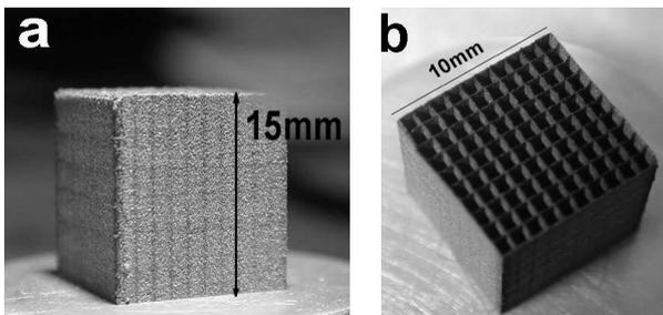
**Fig. 3:** Hollow square prism (steel 1.4404, normal atmosphere. **a:** side view, **b:** top view, showing the grid-like arrangement of the separating walls
