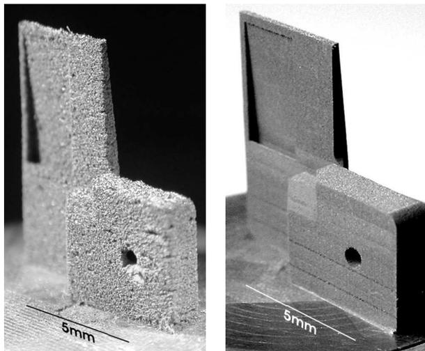
**Fig. 6a:** A fiber positioning tool produced from 80Ni20Cr in normal atmosphere within 90min.
