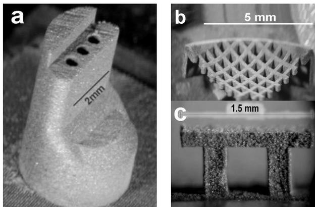
**Fig. 1a:** laser micro sintered grip bit. **b,c:** micro sintered parts with high resolution and  $90^\circ$  undercut angles.
