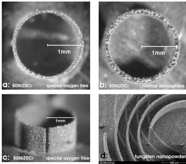
**Fig. 5a,c:** Cylindrical wall generated from 80Ni20Cr in an oxygen free environment with a wall thickness of approximately 60µm. **b:** cylinder from 80Ni20Cr generated under normal atmosphere (wall thickness: 125µm). **d:** coiled tungsten ligament from nanopowder (gauge: 40µm).
