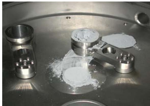
Figure 4 Ringblade serves as rake and powder storage
