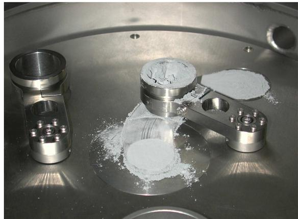
**Figure. 3:** Ringblade serves as rake and powder storage
