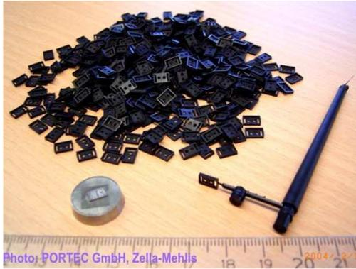
**Fig. 12b:** The laser micro sintered mold remained unaffected after 500 casts with POM
