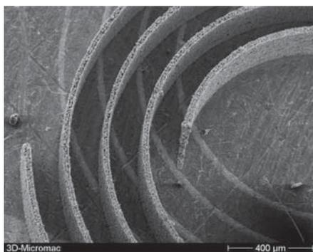
FIGURE 4: Coiled tungsten ligament; gauge 35 µm.
