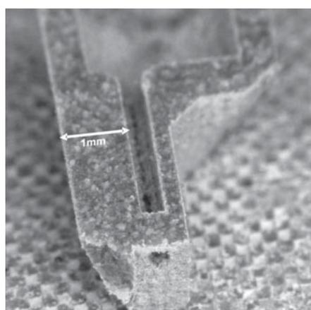
FIGURE 13: Functional component (left), demonstrator part (right) generated by laser micro sintering from oxideceramic powders.
