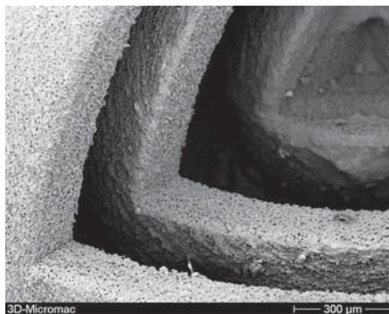
FIGURE 5: Blow-up of three nested spherical shells (see Fig. 6b).
