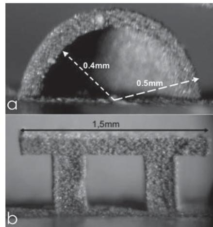
FIGURE 7a,b: Quarter-sphere shell and transverse structure with 90° undercut.
