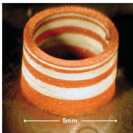
FIGURE 9b: Laser micro sintered part from copper and silver.
