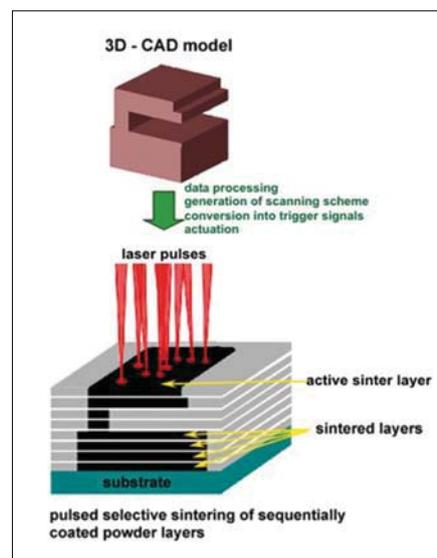
FIGURE 2: Laser micro sintering with separately set pulses.
