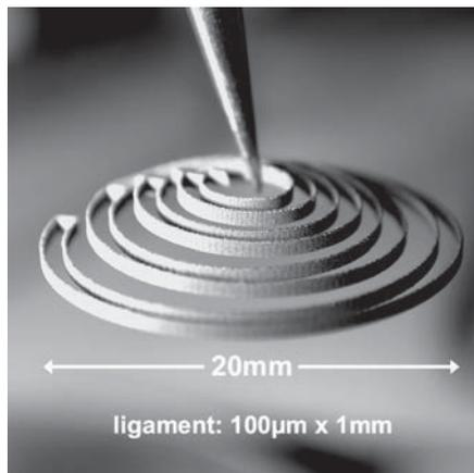
FIGURE 8b: Molybdenum coil, sintered under normal atmosphere.
