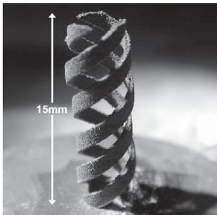
FIGURE 8a: Triplex helix (steel 1.4404) sintered under normal atmosphere; height: 15 mm).
