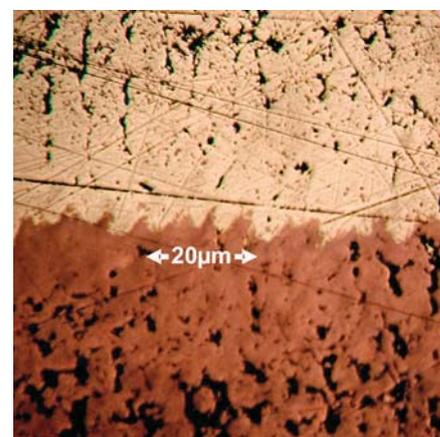
FIGURE 9c: Cross section view of the interface between a copper and a silver section.
