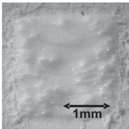
FIGURE 11: Improved laser sinter result after reduction of the glass-phase.
