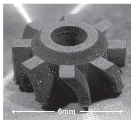
FIGURE 14: Laser micro sintered cog from SiSiC-powder.
