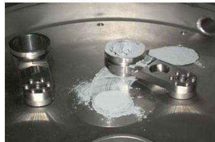
FIGURE 1: Ring blade serves as rake and powder storage.
