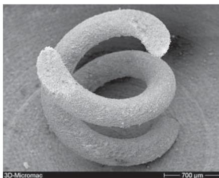
FIGURE 6a: Bi-helical tungsten coil.
