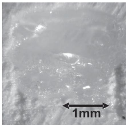
FIGURE 10: First sintering result with too much glass content in the sintered body.
