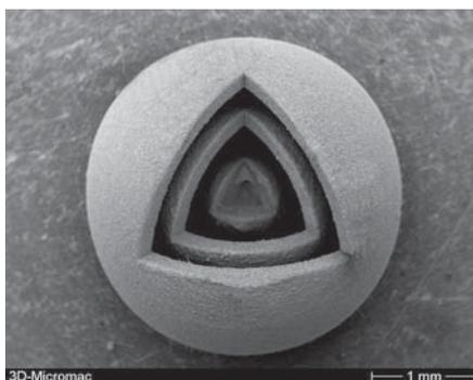
FIGURE 6b: Three nested spherical shells.
