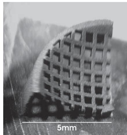
FIGURE 7c: Grid insert with 90° undercut.
