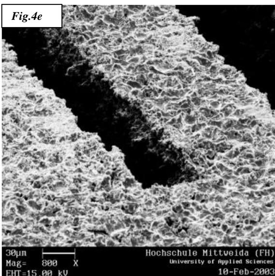
**Figures 4:** SEM views of a multishape test structure sintered of tungsten powder; the diagonal hatch of the surface texture (a) as well as local scourings of the upper surface (d) are due to abrasion by the rake after occasional slight failures of the probe piston. The narrowest achieved notches have a width of 40 μm (c,d,e). The structure is 400 μm high.
