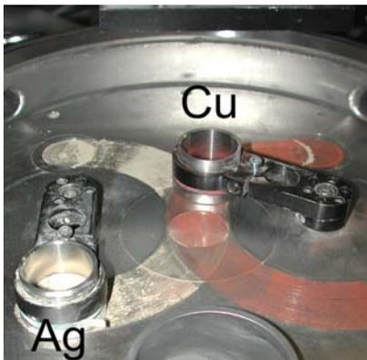
**Fig. 6a:** Automatic change of powders during laser micro sintering.
