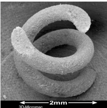
**Fig. 4a:** Double helix from 0.3 micron tungsten powder.
