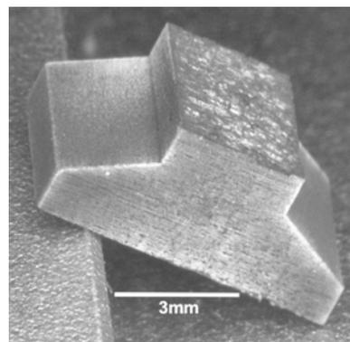
**Fig. 9c:** Miniature from SiC powder (sintered under shield gas).
