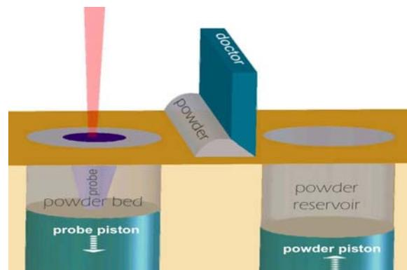
**Fig. 1:** Schematic of selective laser sintering.
