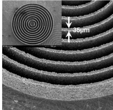
**Fig. 3b:** Top view of tungsten ligaments showing the cut-ins from the pulses.
