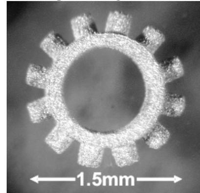
**Fig. 5c:** Cogged wheel; (2 micron silver powder; normal atmosphere). Courtesy of JOTEC GmbH, Stuttgart
