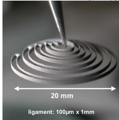
**Fig. 5b:** Elastic coil (7 micron molybdenum powder; normal atmosphere).
