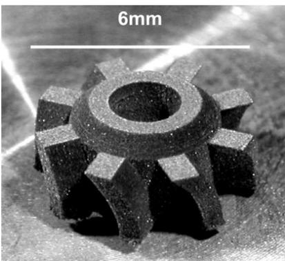
**Fig. 9a:** Laser sintered gear wheel from SiSiC without infiltration (normal atmosphere).
