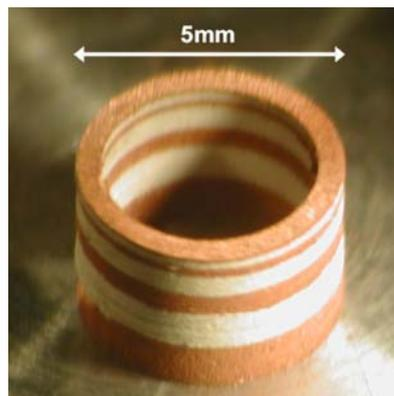
**Fig. 6b:** Cylinder with alternating segments of copper and silver.
