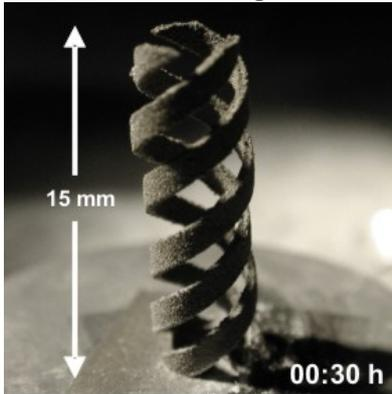
**Fig. 5a:** Triple helix (10 micron stainless steel powder; normal atmosphere; 30 min process).
