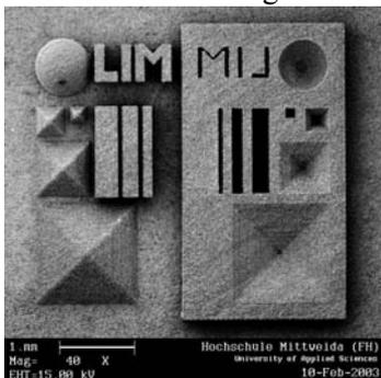
**Fig. 2a:** Multi shape test structure from 0.3 micron tungsten powder.
