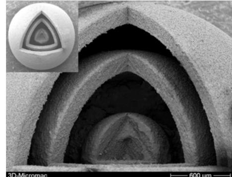
**Fig. 3c:** Blow up view of a specimen consisting of three nested spheres.
