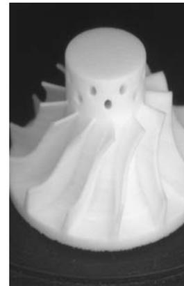
**Fig. 8a:** Laser micro sintered miniature impeller from alumina-ceramics. Courtesy of EOS GmbH, Munich
