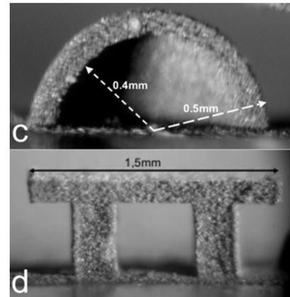
**Fig. 4c,d:** Quarter-sphere shell and traverse structure.
