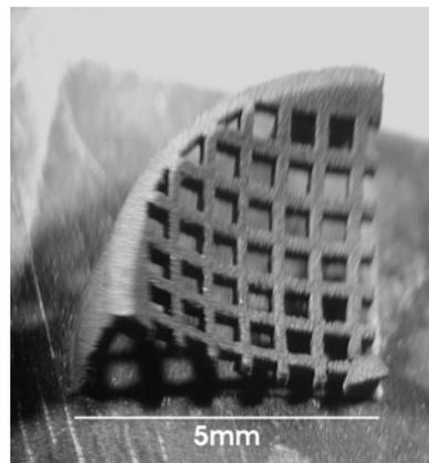
**Fig. 4b:** Tungsten grid generated with unlimited undercuts.
