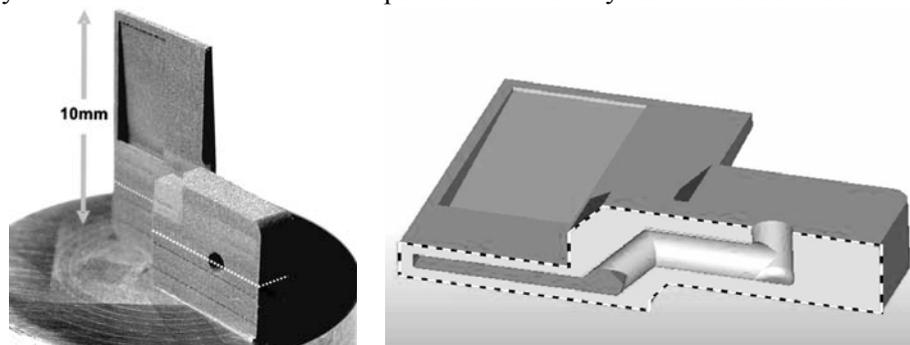
**Figs. 2b:** First functional part (wafer positioner) from 3 micron tungsten powder. The drawing on the right shows a cross section along the dotted line in the photograph on the left. The hidden channel is visible.
