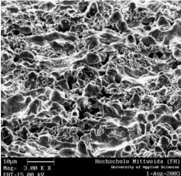
**Fig. 3a:** Surface of a laser micro sintered specimen. Minimal roughness  $r_a = 1.5 \mu\text{m}$ .
