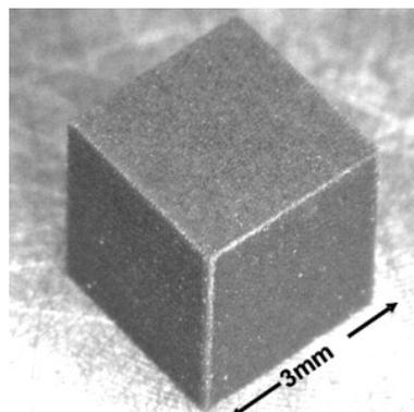
**Fig. 9b:** Cube from SiSiC (normal atmosphere).
