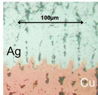
**Fig. 6c:** Fusion zone between a sintered copper and the succeeding silver segment.
