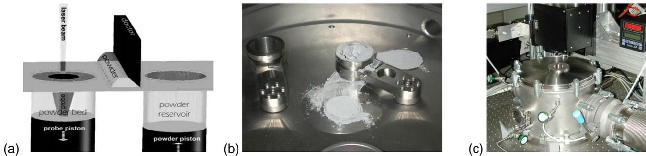
Figure 1: (a) Schematic of a laser sintering device; (b) doctor substituted by cylinder; (c) vacuum tight casket.
