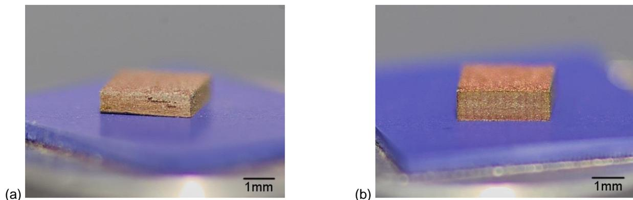
Figure 2: (a) copper block sintered onto LTCC with a “two-fold line-scan” strategy; (b) copper block, firmly attached to the LTCC-substrate via the “square-array” strategy.
