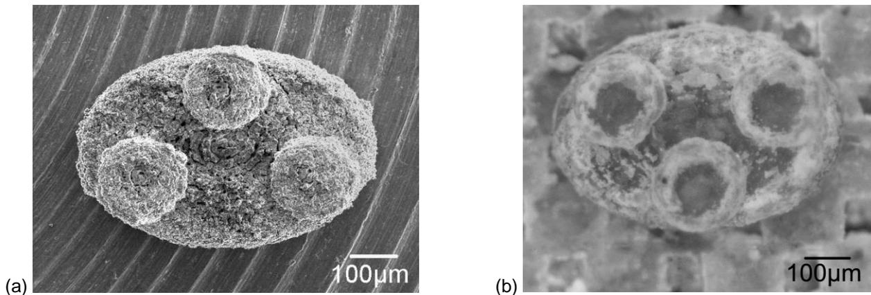
Figure 8: Comparison of the material dependent resolutions (a) Mullite/molybdenum cermet. (b) Mullite-ceramic.
