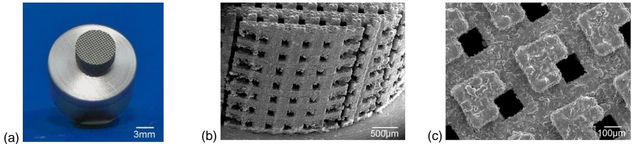
Figure 6: (a) Micropart from a stainless steel (1.4404) powder, blended with TaC. (b,c) Detail SEM views.
