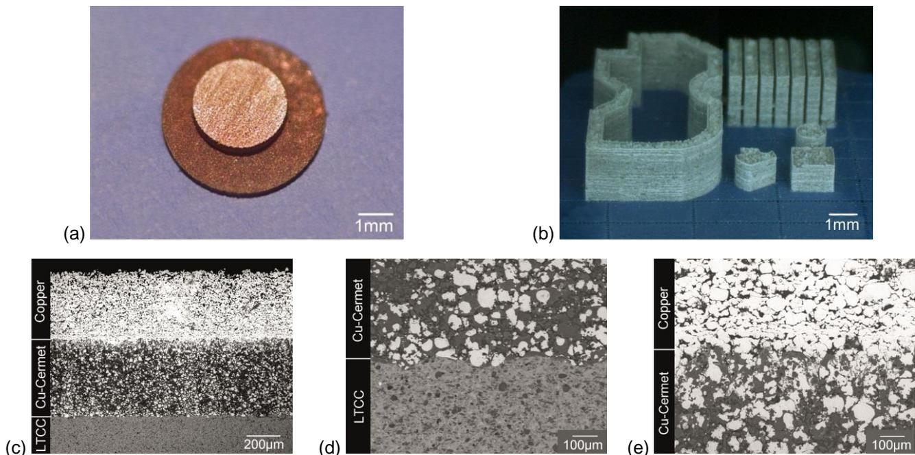
Figure 3: (a) triple sandwich of LTCC (bottom) / Cu-cermet / Cu (top). (b) laser sintered mullite-ceramics (grey) attached to LTCC (blue). (c-e) Cross section views of the interfaces in the triple sandwich LTCC/Cu-cermet/Cu.
