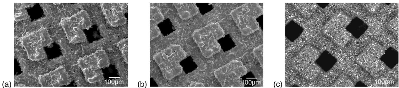
Figure 7: SEM recordings of microparts with the same design, generated from three different materials .(a) NiCr/Mo (b) Steel 1.4404/TaC(c) mullite/molybdenum cermet.
