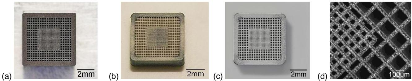
Figure 5: Micro grids of mullite/molybdenum cermet after various stages of tempering at 800 °C. (a) Un-tempered (b) After 1 h. (c) After 6 h. (d) Detail SEM micrograph of the as laser sintered specimen.
