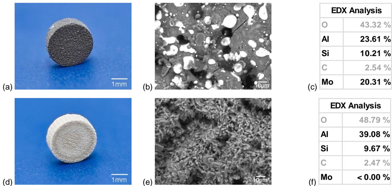
Figure 4: (a) Laser sintered body of mullite/molybdenum cermet with a weight ratio of 75:25. (b) Surface SEM view of the body, as sintered. (c) EDX analysis of the material as sintered. (d) Specimen after additional tempering at 1650 °C. (e) Surface SEM view of the body after additional tempering. (f) EDX analysis of the specimen (results in at %) after additional tempering.
