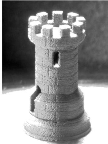
**[Fig. 11d]:** Specimen that had been laser sintered with low fluence after subsequent oven sintering.
