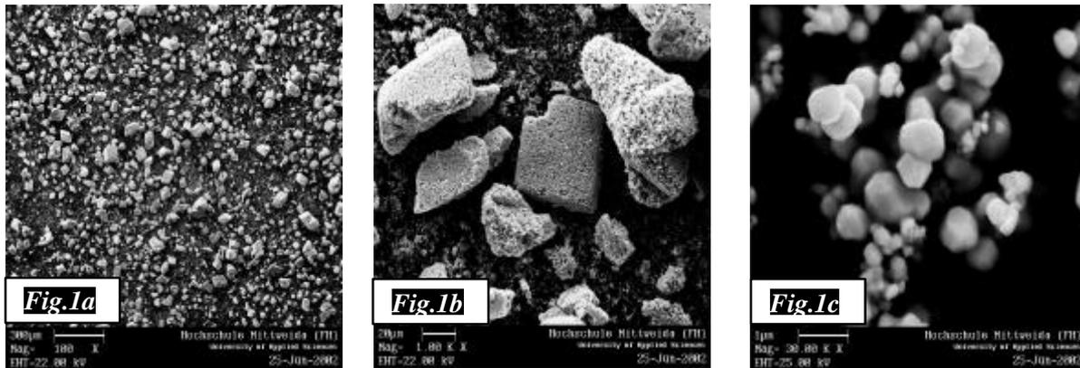
***Figures 1: SEM views of tungsten powder with an average grain size of  $0.3\mu\text{m}$  at different magnifications.***
