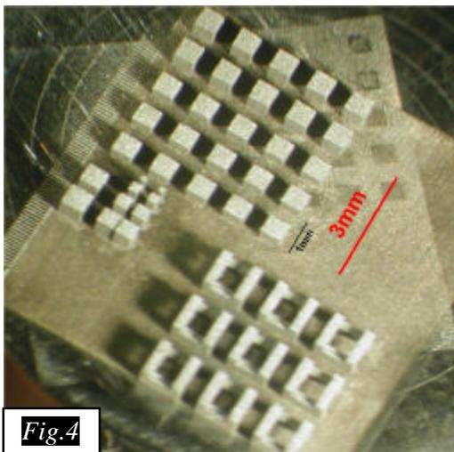
**Figure 4:** Array of tungsten cuboids and bridges, firmly attached to the substrate.
