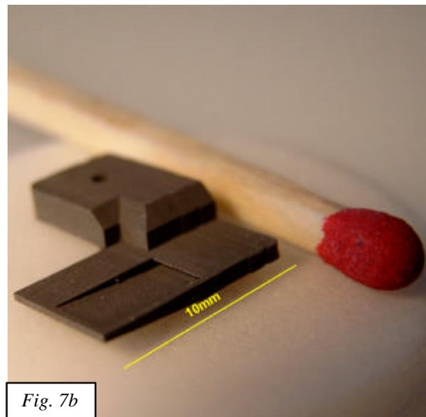
**Figures 7:** *A functional freeform was generated, loosely attached to a stainless steel substrate (a). The freeform was disassembled easily from the substrate.*
