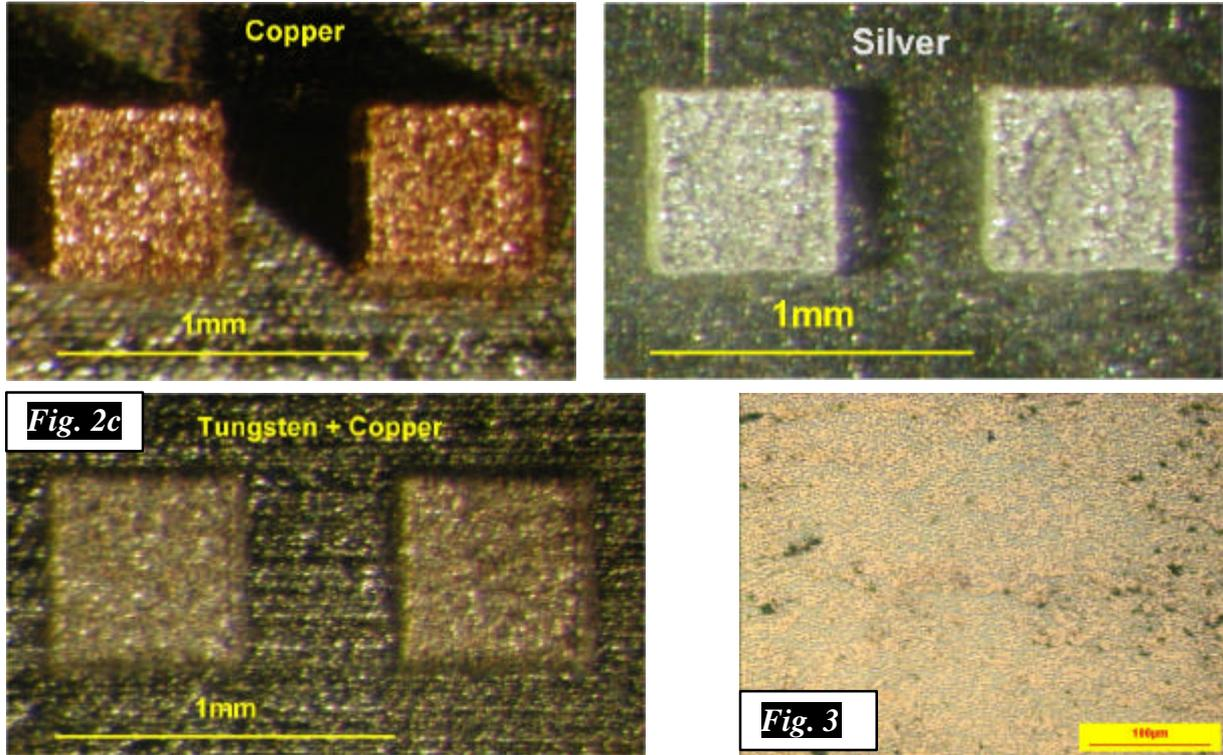
**Figures 2:** Cuboids sintered from metal powder: copper (a), silver (b) and copper/tungsten(c).
