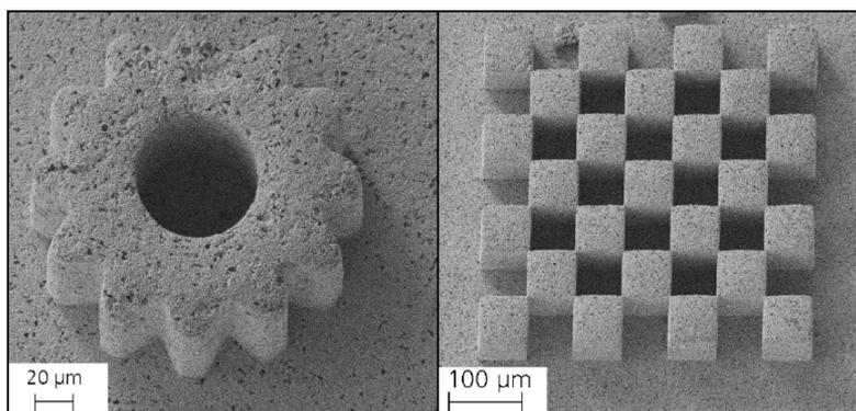
*Fig. 1:  $\mu$ -MIM parts made of WCu20:*
