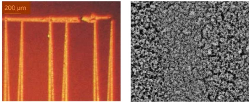
Fig. 6: Sputtered powder layers of gold; porous structure ( $p = 1.5\text{mbar}$ ,  $d = 6250\text{nm}$ ,  $t = 300\text{s}$ ) as in Fig 3b, with sintered tracks:
