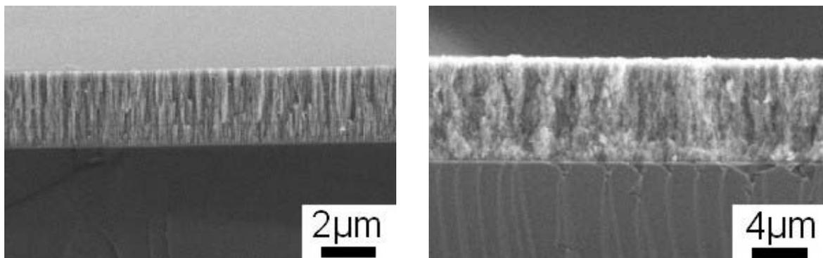
*Fig. 5: Sputtered powder layers made of WCu20 under different argon pressure atmospheres:*
