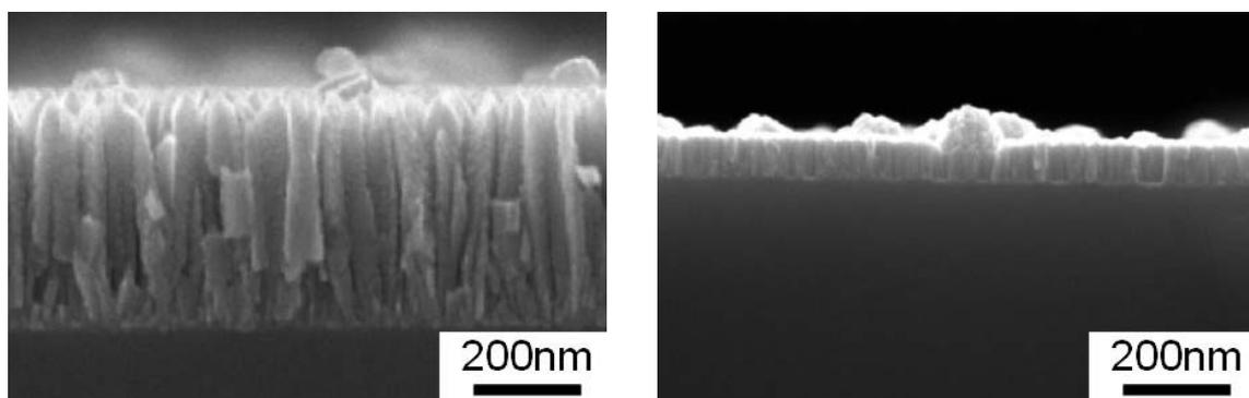
*Fig. 4: Sputtered powder layers made of copper under different argon pressure atmospheres:*
