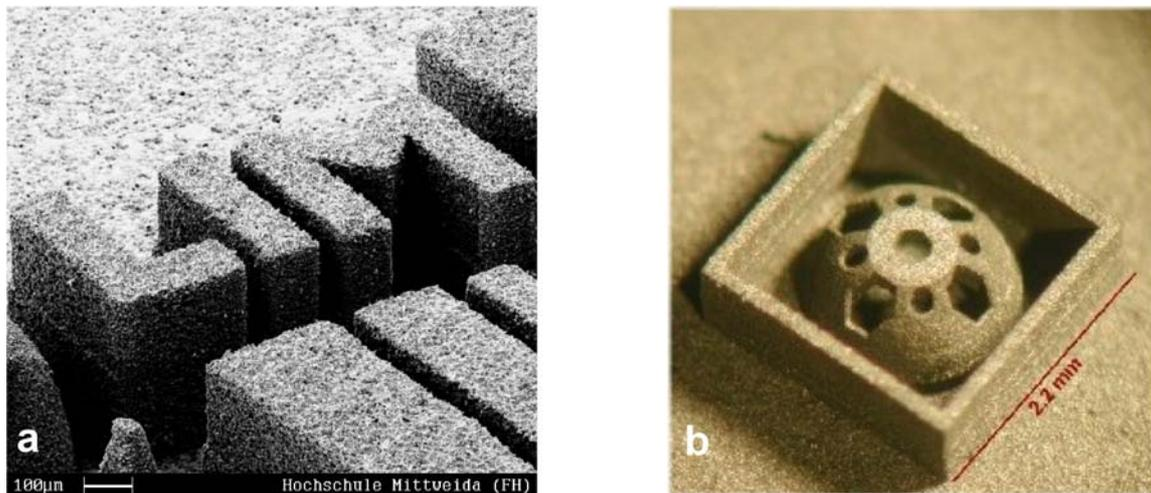
*Fig. 2: Laser micro sintering products from a single component powder*
