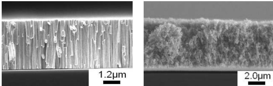
*Fig. 3: Sputtered powder layers made of gold under different argon pressure atmospheres:*
