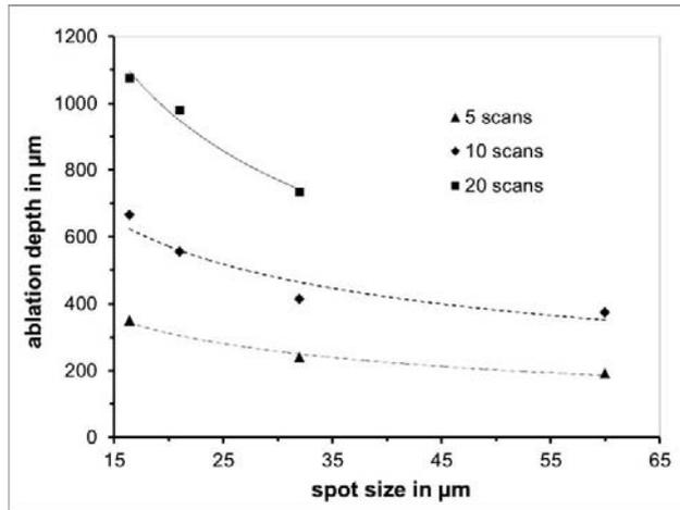
Figure 6: Ablation depth vs. number of scans at different spot sizes, parameters:  $P_{cw} = 2.65$  kW,  $v_{sc} = 600$  m/min.
