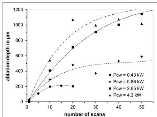
Figure 2: Ablation depth vs. number of scans for various laser power levels, parameters:  $d_{86} = 21 \text{ }\mu\text{m}$ ,  $v_{sc} = 900 \text{ m/min}$ .
