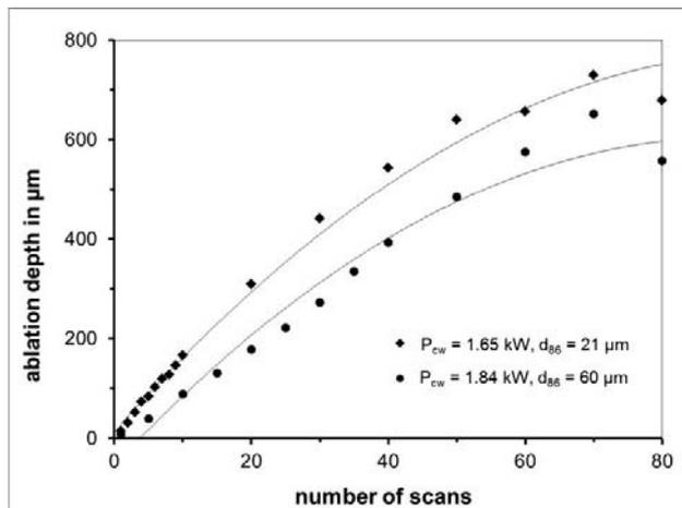
Figure 7: Ablation depth vs. number of scans for two spot sizes, parameters:  $P_{cw} = 1.65$  kW and  $P_{cw} = 1.84$  kW,  $v_{sc} = 2250$  m/min and  $v_{sc} = 2400$  m/min.
