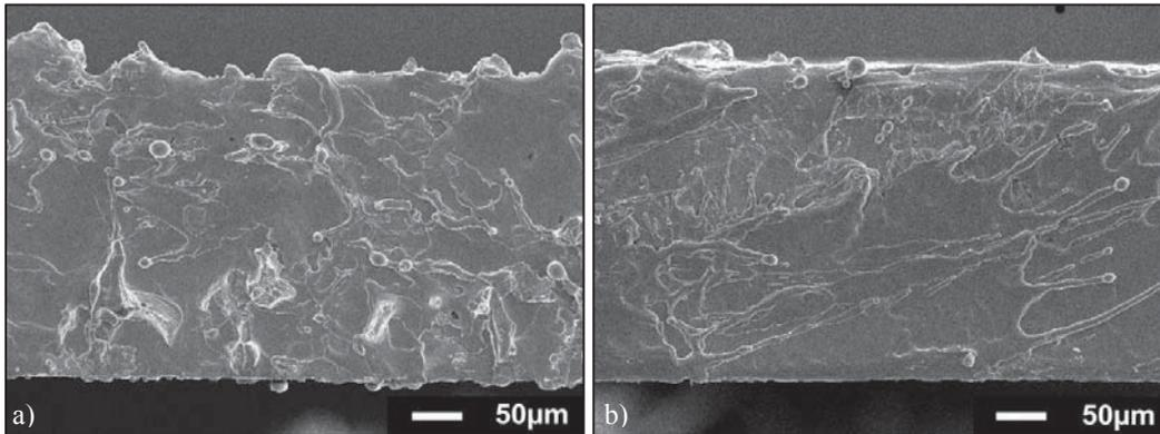
Figure 9: SEM micrographs of cutting edges, parameters:  $d_{86} = 21 \mu\text{m}$ ,  $v_{sc} = 600 \text{ m/min}$ , sheet thickness 0.3 mm, a)  $P_{cw} = 0.62 \text{ kW}$ , 28 scans; b)  $P_{cw} = 1.76 \text{ kW}$ , 6 scans.
