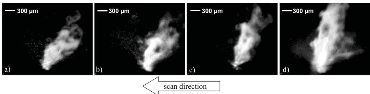
Figure 12: Highspeed camera recordings at various scan speeds, parameters:  $P_{cw} = 1.7 \text{ kW}$ ,  $d_{86} = 21 \mu\text{m}$ ,
