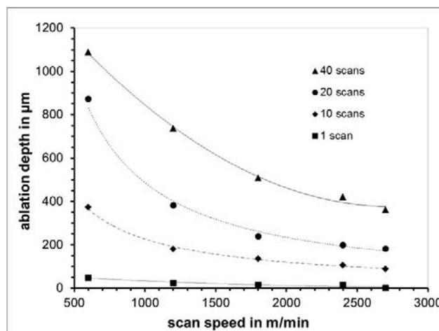
Figure 4: Ablation depth vs. scan speed for different number of scans, parameters:  $P_{cw} = 2.65$  kW,  $d_{86} = 60$   $\mu\text{m}$ .
