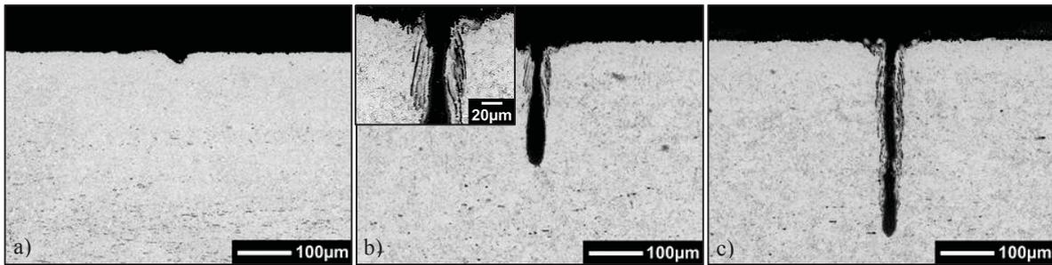
Figure 1: Cross section photographs of cutting kerfs obtained with various number of scans, parameters:  $P_{cw} = 0.86 \text{ kW}$ ,  $d_{86} = 21 \text{ }\mu\text{m}$ ,  $v_{sc} = 1200 \text{ m/min}$ ; a) 1 scan, b) 10 scans, c) 20 scans.
