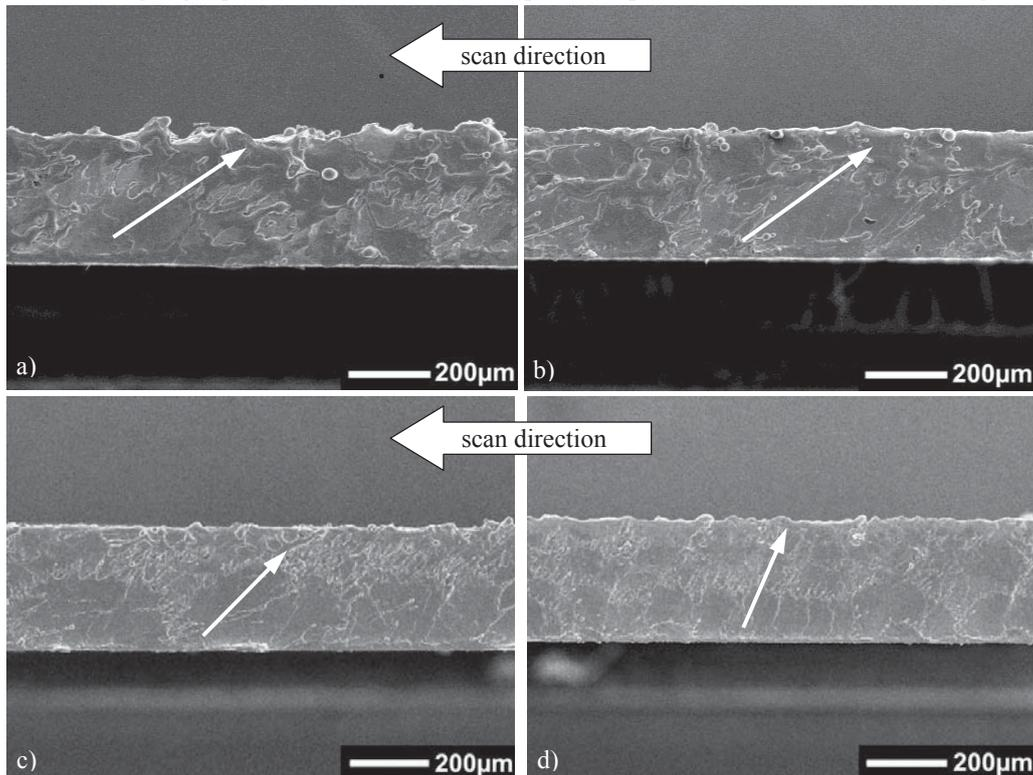
Figure 10: SEM micrographs of cutting edges for various scan speeds, parameters:  $P_{cw} = 0.94 \text{ kW}$ ,  $d_{86} = 32 \mu\text{m}$ , a)  $v_{sc} = 480 \text{ m/min}$ , 8 scans, b)  $v_{sc} = 600 \text{ m/min}$ , 9 scans, c)  $v_{sc} = 900 \text{ m/min}$ , 13 scans, d)  $v_{sc} = 1800 \text{ m/min}$ , 22 scans.
