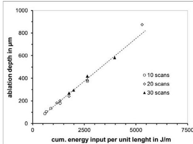
Figure 3: Ablation depth vs. cumulated energy input per unit length for various number of scans, parameters:  $P_{cw} = 2.65$  kW,  $d_{86} = 60$   $\mu\text{m}$ , varied scan speed.
