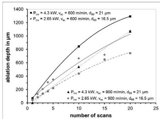
Figure 5: Ablation depth vs. number of scans for a given intensity of laser radiation of  $2.5 \cdot 10^9$  W/cm<sup>2</sup> realized with different combinations of spot size and applied laser power for scan speeds of 600 m/min and 900 m/min.
