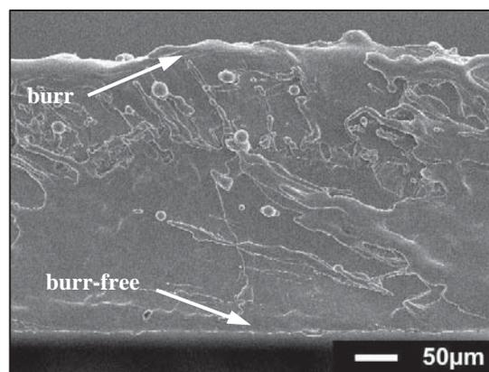
Figure 8: SEM micrograph of the cutting edge, parameters:  $P_{cw} = 1.8$  kW,  $d_{86} = 16.5$   $\mu\text{m}$ ,  $v_{sc} = 600$  m/min, 5 scans.
