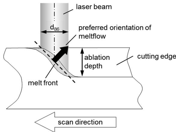
Figure 11: Schematic of the melt front formation in laser ablation cutting.
